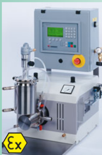
DISPERMAT® SL-C Ex Power: 1,1 - 4 kW Milling chamber volume: 50-2000ml Millbase quantity: 50 ml – 50 l C Technology
