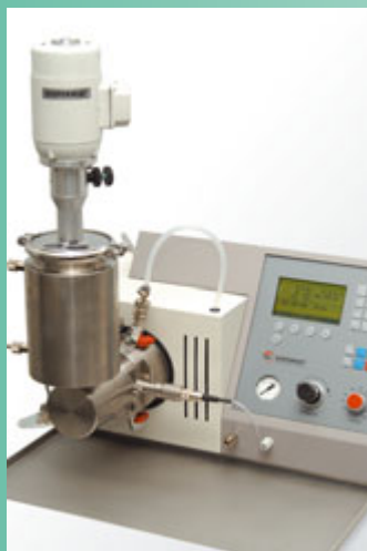
DISPERMAT® SL Power: 1,1 - 4 kW Milling chamber volume: 50-2000ml Millbase quantity: 50 ml – 50 l M + C Technology
